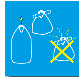
Only use lifting forks with rounded edges
